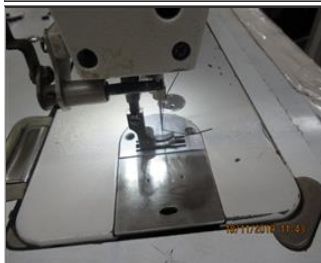
Photo of non-conformity Sewing machine missing finger guard.JPG
