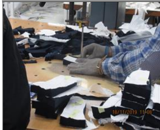
Photo of the personal protection equipments (if applicable) Cutting worker wearing steel mesh gloves.JPG
