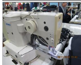
Photo of non-conformity Sewing machine missing eye guard.JPG
